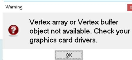
It is necessary to changes the graphical configuration. Go to **Start >> Programs >> Iber >> Iber Safe Mode** menu.
